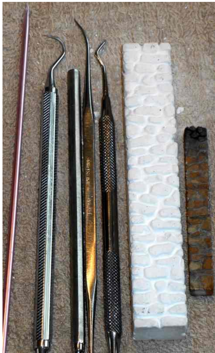
Picture 19: Tools used to carve plaster.
